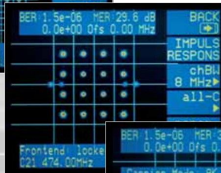
Constellation diagram of an OFDM signal (16QAM)
